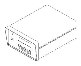
The VA-2000 is a stand-alone desk top unit. It operates from a nominal 12 volt DC. A UL listed wall mount transformer is supplied for primary power. Optionally, an internal battery backup may be installed. A VA-2000 must be ordered with a radio receiver and antenna. Four different versions are offered, as follows:
