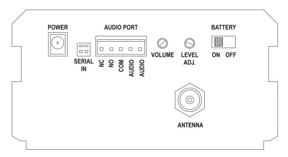
In addition, a number of optional features may be present. These include a relay closure and an audio output path through a five position "AUDIO" connector, as part of the Audio Output option, plus "LEVEL" and "VOL." controls for audio. For the Battery Back-up option, a "BATTERY ON OFF" switch and a "CHARGER POWER" connector are included.
